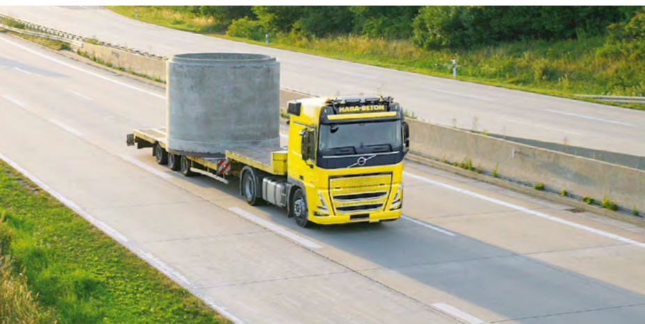
A shaft ring is being transported to the building site.
