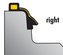
Control correct fitting of the seal against shoulder of spigot end. Control correct seat of the load transfer hose in the middle of the spigot end front.
