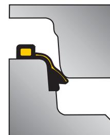
Do not use any lubricant on the seal or on the socket!
